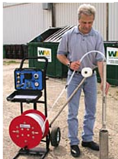
Low Flow Double Valve Pump Setup in Field
